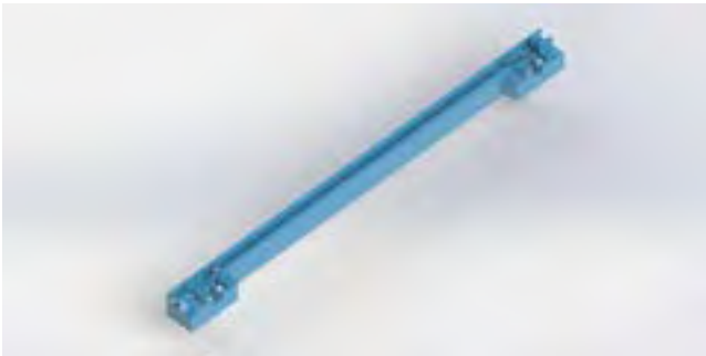
Board guides rail
