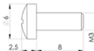
Ph. cross recessed countersunk screw M3x8
